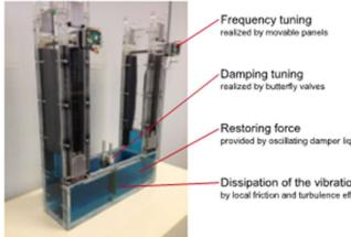
provided by oscillating damper liquid
